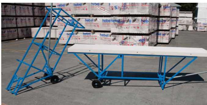
Figure 4.2.2 Hebel Panel Trolleys for easier and safer handling and cutting of Hebel PowerPanels.
