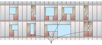
Poor panel layout results in complex on-site cutting of panels
