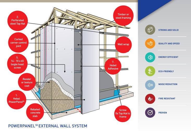
The PowerPanel<sup>50</sup> system consists of 50mm thick, steel-reinforced AAC panels, vertically secured to the structural frame via horizontal perforated top hat sections. The wall is then rendered with a recommended coating system – providing a faster way of constructing external facades for residential builds.
