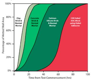
Note: Test procedure in accordance with BS4315 Part 2, 1970; Methods of Test for Resistance to Air and Water Penetration. Tested at CSR Building Materials Research Laboratory, November 1989
