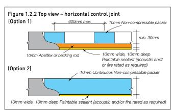
NOTE: Use 10mm wide by 10mm deep CSR Fireseal Sealant at vertical and horizontal control joints to achieve FRL of 90/90/90 for the wall system. See section 1.5. Protect Fireseal Sealant from rain until sealant has developed a thick skin. Once cured, Fireseal should be painted over with a compatible external grade acrylic coating i.e Dulux Acratex or similar.
