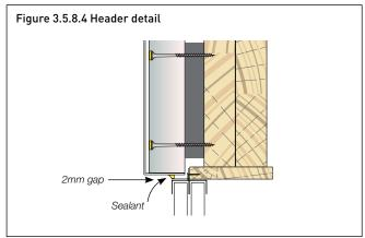
NOTE: Drainage of window and door sills, in either aluminium or timber, should be directed to the outside of the building, on top of the window sill.
