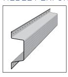
Hebel Perforated Top Hats in galvanised steel are provided in nominal widths of 24mm and 35mm and have been designed and constructed in accordance with AS 3623 and AS/NZS 4600 (NCC Performance Requirement). The following tables are based on 15mm RONDO M515 top hat, 24mm and 35mm Hebel perforated top hat section.
