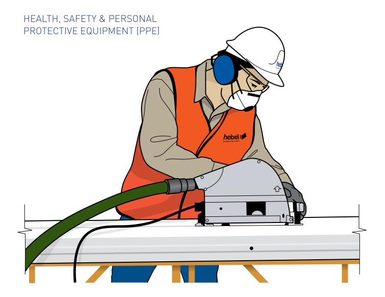
Use PPE gloves and wear suitable clothing when handling Hebel panels and blocks. Hebel products are cement-based, and though the dust is not absorbed through the skin it may cause irritation – particularly in association with heat and sweat. Repeated heavy contact with the dust can result in skin rash, called dermatitis, which typically affects the hands. To minimise exposure to dust on your skin we recommend wearing gloves (standard duty leather or equivalent AS 2161).
