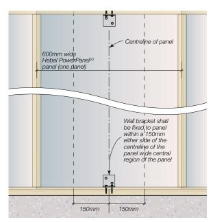
NOTE: GROUND LEVEL: Screw fix wall bracket at top and bottom plates of wall frame and to the PowerPanel<sup>50</sup> panel. No brackets are required at bottom plate when using a continuous deflection head track or continuous steel angle for base connection.
