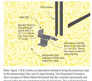
to the bottom plate/ floor joist in steel farming. This fixing detail involves a short cut piece of 50mm Hebel Perforated Top Hat, oriented transversely and placed within the top and bottom track of steel frame. The wall bracket fixed to top hat and to the steel frame shall be fixed to panel within a 150mm either side of the centreline of the panel wide central region of the panel.
