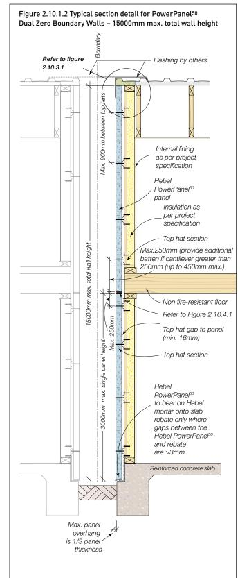
NOTE: A maximum Hebel wall height of 3,900mm can be constructed with a horizontal Hebel Adhesive joint between the upper and lower Hebel panels for areas that contain heights above 3,000mm. The maximum length of Hebel PowerPanel<sup>50</sup> is 3,000mm, therefore the lower panel can be installed as a max length panel vertically, with either a horizontal 600mm wide panel (max total wall height 3,600mm) or a vertical 900mm high panel (max total wall height 3,900mm).
