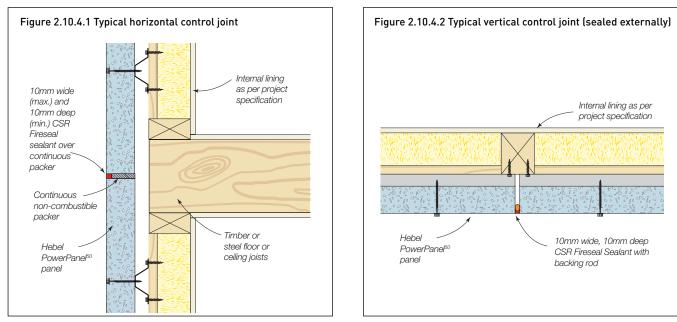
NOTE: Where access to the external Hebel face available, both vertical and horizontal control joints are to be sealed to the external face of the Hebel panels (as shown in Figure 2.10.4.2). Where access to the external Hebel face is not available, both vertical and horizontal control joints are to be sealed to the internal face of the Hebel panels. Figure 2.10.4.1 is shown for loadbearing wall frame. For non-loadbearing wall frames, please contact Technical team for further information.
