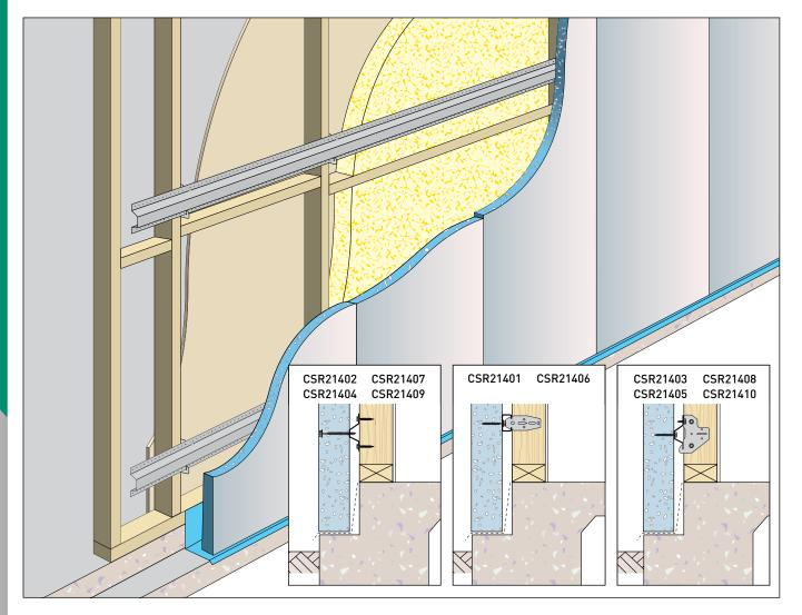
Table 2.1.1 PowerPanel<sup>50</sup> Dual Zero Boundary Wall Systems
