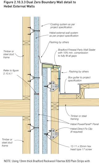
NOTE: Using 13mm thick Bradford Rockwool Fibertex 820 Plain Strips with density of 110kg/m<sup>3</sup> at horizontal control joint is applicable for Dual Zero Boundary Walls when the horizontal control joint is not exposed to outside weather conditions when the top of the wall is capped with flashing between boundary.
