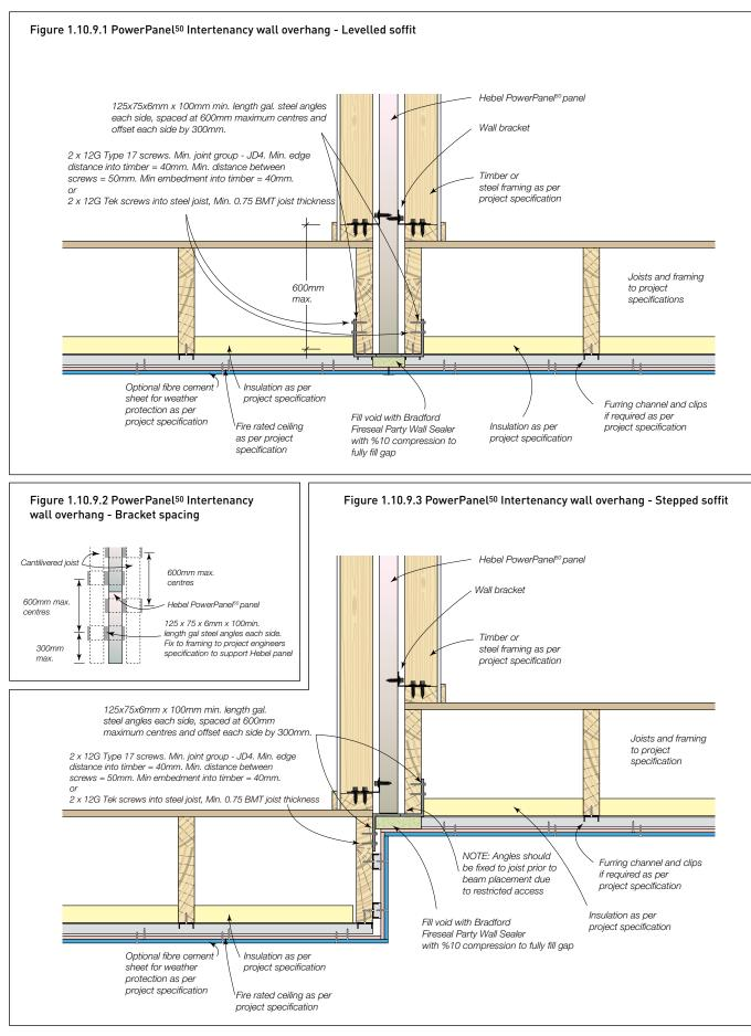
Note: The maximum allowable wall height for Figures 1.10.9.1 and 1.10.9.3 is 6m.
