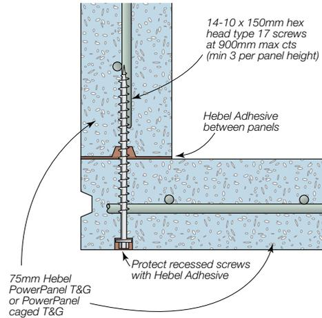
**Figure 3.6.2.5 Hebel Intertency to Corridor wall junction**
