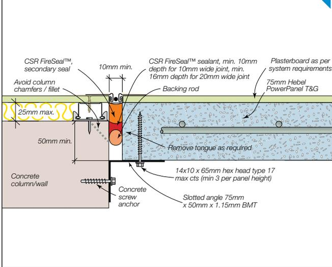
Figure 3.6.2.8 Offset panel to column with CSR FireSeal™ fillet
