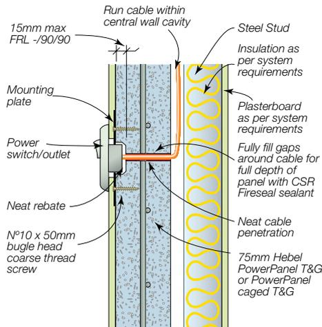
Figure 3.6.6.9 Power switch / outlet installation to steel stud or furring channel
