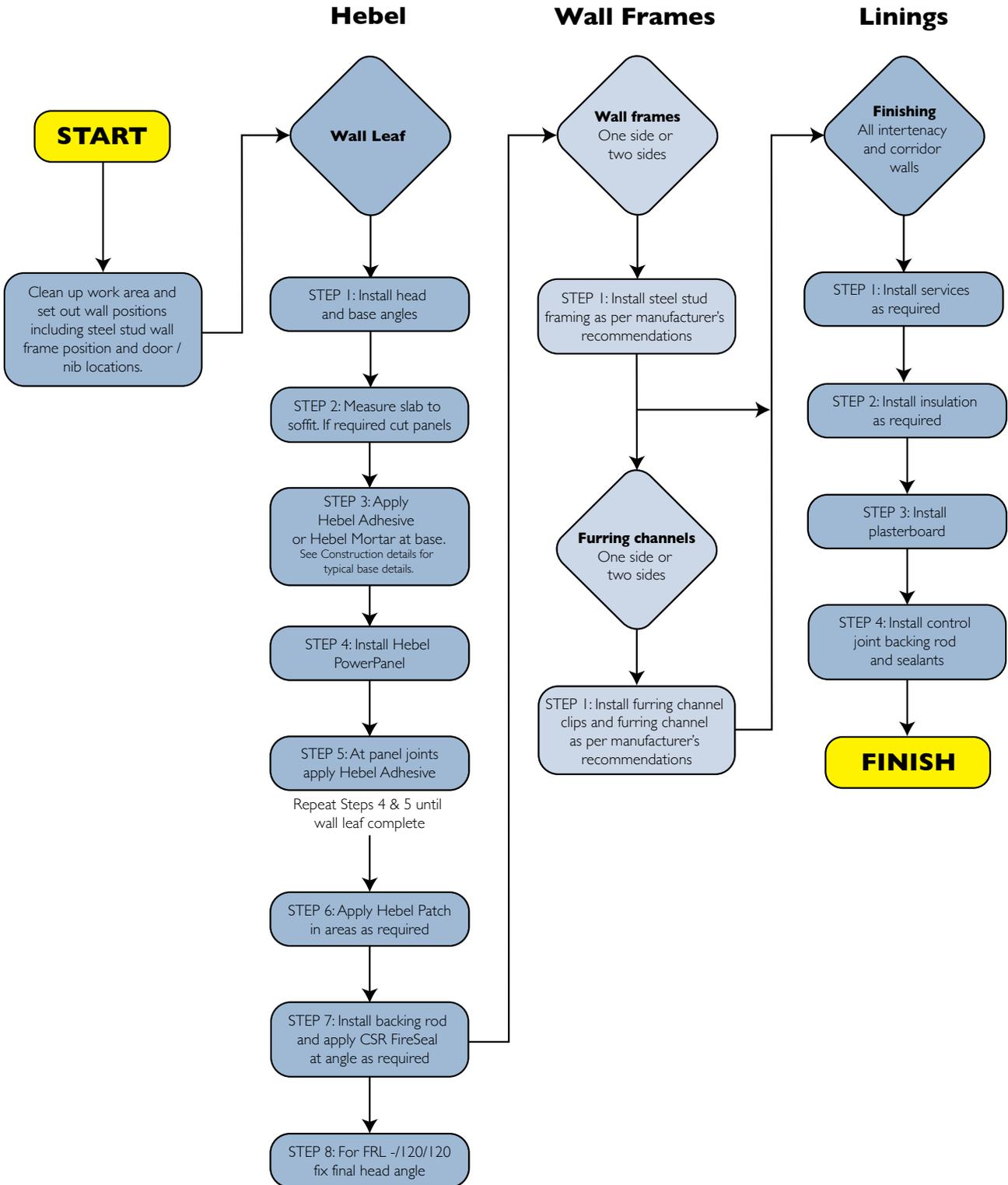
Figure 3.1.2 Shaft and services wall systems - vertical and horizontal installation
