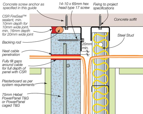
Figure 3.6.6.11 Fire damper penetration
