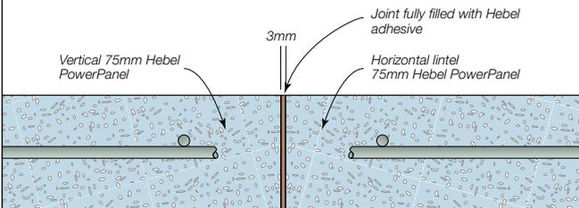
**Figure 3.6.4.4 Lintel junction detail with 50mm seating - SECTION AA**
