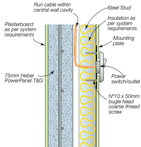
Figure 3.6.6.10 Cable installation within the cavity for switch / outlets located on both sides of wall
