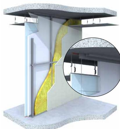
The Hebel Express Head system simplifies design and construction and minimises risk. The Hebel PowerPanel is installed from slab to soffit with only one fire sealant position required at head.
