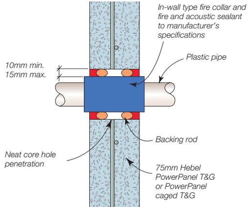
Figure 3.6.6.13 Plastic pipe penetration with wall mounted fire collar
