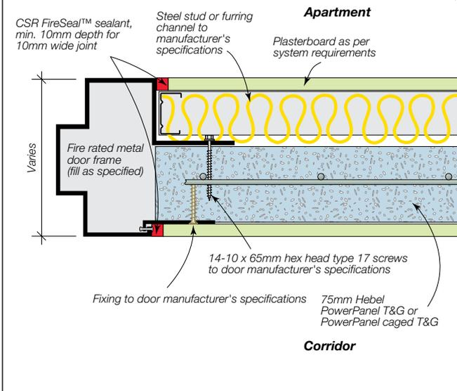
**Figure 3.6.4.8 Hebel Intertency wall to corridor at door frames**
