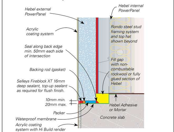
**Figure 3.6.3.3 Hebel Intertency / Corridor Wall to brick veneer junction**
