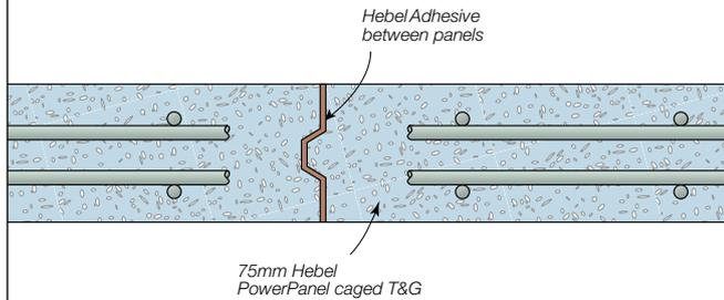
**Figure 3.7.3.2 Splay corner junction for vertical panel installation only**
