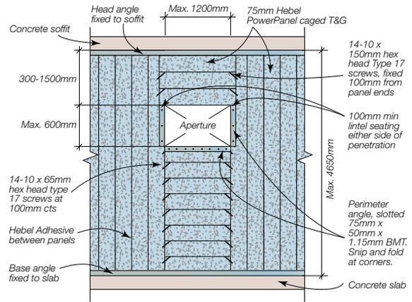
Adjust width of lintels 100mm each side of penetration
