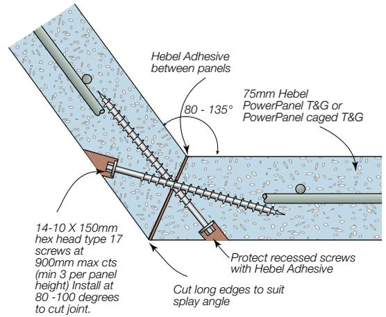
**Figure 3.6.2.3 Panel to column junction**
