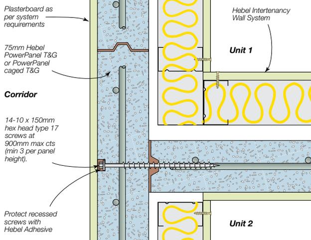
**Figure 3.6.2.6 Panel side to panel overlap junction**
