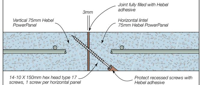
**Figure 3.6.4.5 Optional square edge panel connection detail with no seating and skewed screws**
