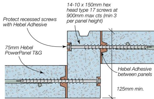
Figure 3.6.2.7 Offset panel to column detail for FRL -/60/60
