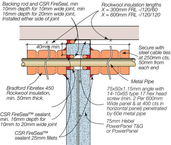
**Figure 3.6.6.4 Metal pipe penetration**
