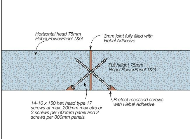
**Figure 3.6.4.6 Door nib detail for widths 100-300mm - SECTION BB**
