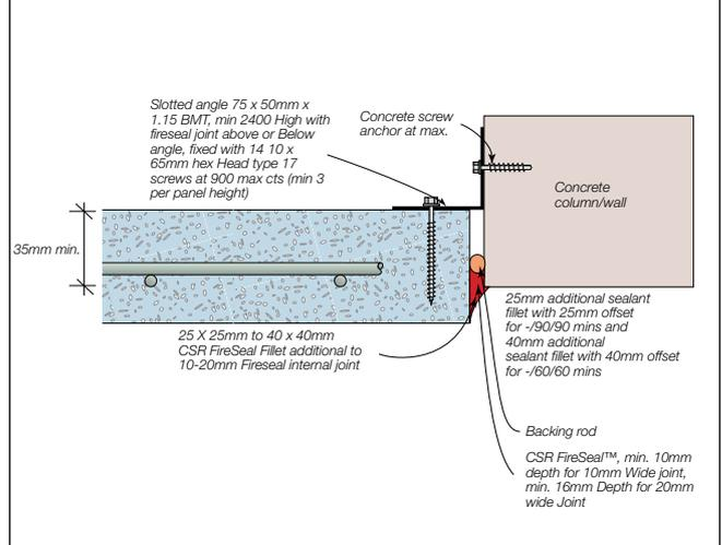
Figure 3.6.2.9 Offset panel to column with CSR FireSeal™ fillet
