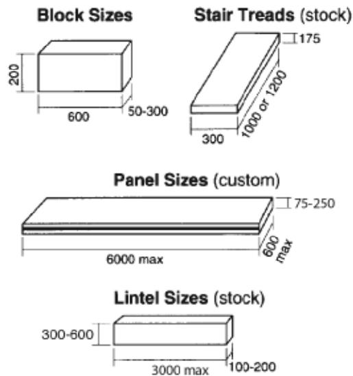
**Table 2.1: Product Range for CSR Hebel Blocks, Lintels & Stair Treads**
