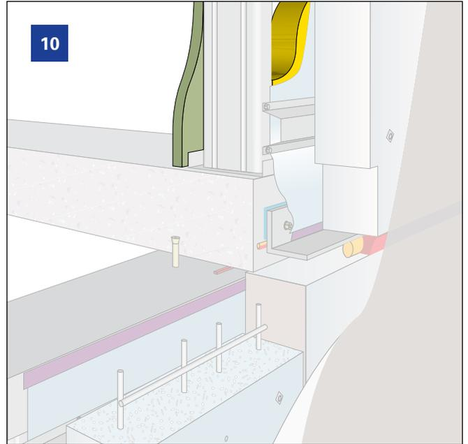
Install Bradford insulation and line internally with Gyprock plasterboard as per the system requirements.
