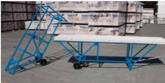
Figure 5.2.2 Hebel Panel Trolleys for easier and safer handling and cutting of Hebel PowerPanels.
