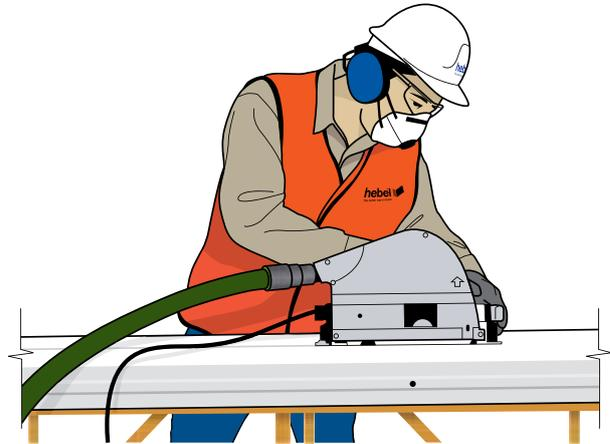
Use PPE gloves and wear suitable clothing when handling Hebel panels and blocks. Hebel products are cement-based, and though the dust is not absorbed through the skin it may cause irritation – particularly in association with heat and sweat. Repeated heavy contact with the dust can result in skin rash, called dermatitis, which typically affects the hands. To minimise exposure to dust on your skin we recommend wearing gloves (standard duty leather or equivalent AS 2161).
