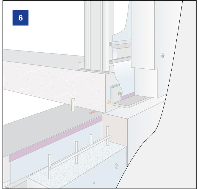
Apply base levelling coat across panel and joints.
