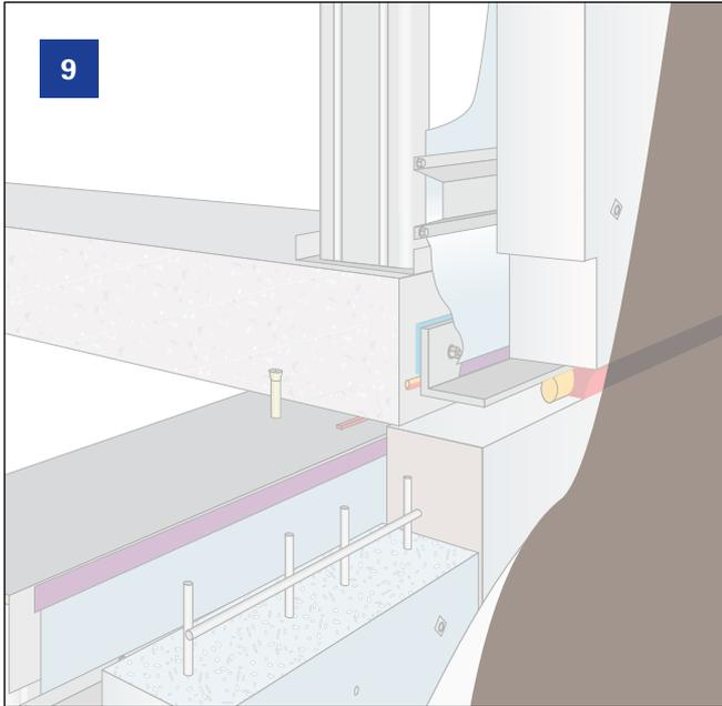
Apply final weatherproofing topcoat by nap roller over the entire area including the control joints providing colour uniformity across the panel and joints.
