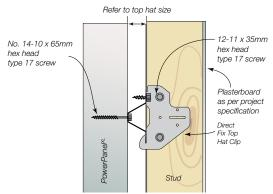
**IMPORTANT:** Top hat clip is fixed on the left hand side of the stud (when looking from inside to the outside of the building) except at the last stud, only, when the clip may be installed upside down.
