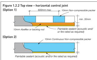
NOTE: Use 10mm wide by 16mm deep CSR Fireseal or Fireblock XT Sealant at vertical and horizontal control joints to achieve FRL of -/120/120 for the wall system. See Section 2.2. Protect CSR Fireseal Sealant from rain until sealant has developed a thick skin. Once cured, CSR Fireseal should be painted over with a compatible external grade acrylic coating i.e. Dulux AcraTex or similar.
