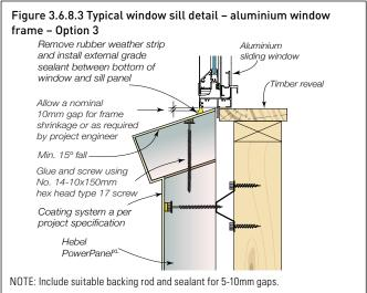
NOTE: CSR Hebel recommends the removal of the rubber weather strip at the window sill prior to applying external grade sealant between the bottom of the window sill and panel. Windows shall be caulked around all sides to ensure that the system remains sealed and not allow water ingress into the cavity. The installation of any alternative details shall be the responsibility of the builder to provide supporting evidence that it meets the requirements of a sealed system and maintains a dry cavity.
