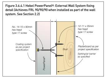
NOTE: When positioning the stud frames allow 5-7mm extra cavity width for the sheet bracing between top hat and timber stud.
