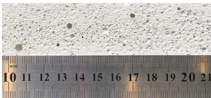
Cross section of AAC, showing the voids.
